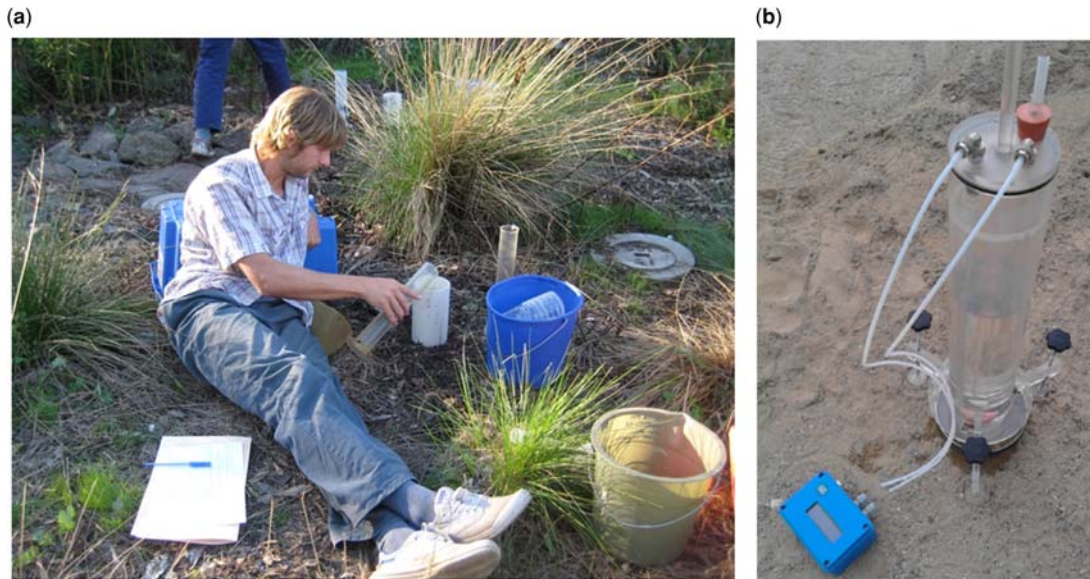
Figure 4.16 (a) example application of single-ring infiltration testing using laborious manual measurement or, (b) automated systems. Sources: (a) Peter Poelsma (University of Melbourne); (b) Simone Di Prima (Università degli Studi di Palermo).
