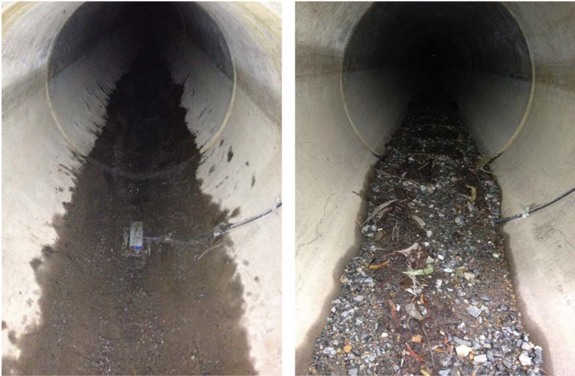
Figure 4.4 Example of a flowmeter being covered by sediments after a storm event, leading to loss of reliable data. In this case sediment accumulation was due to the construction of a small weir downslope of the probe. Source: Peter Poelsma (University of Melbourne).
