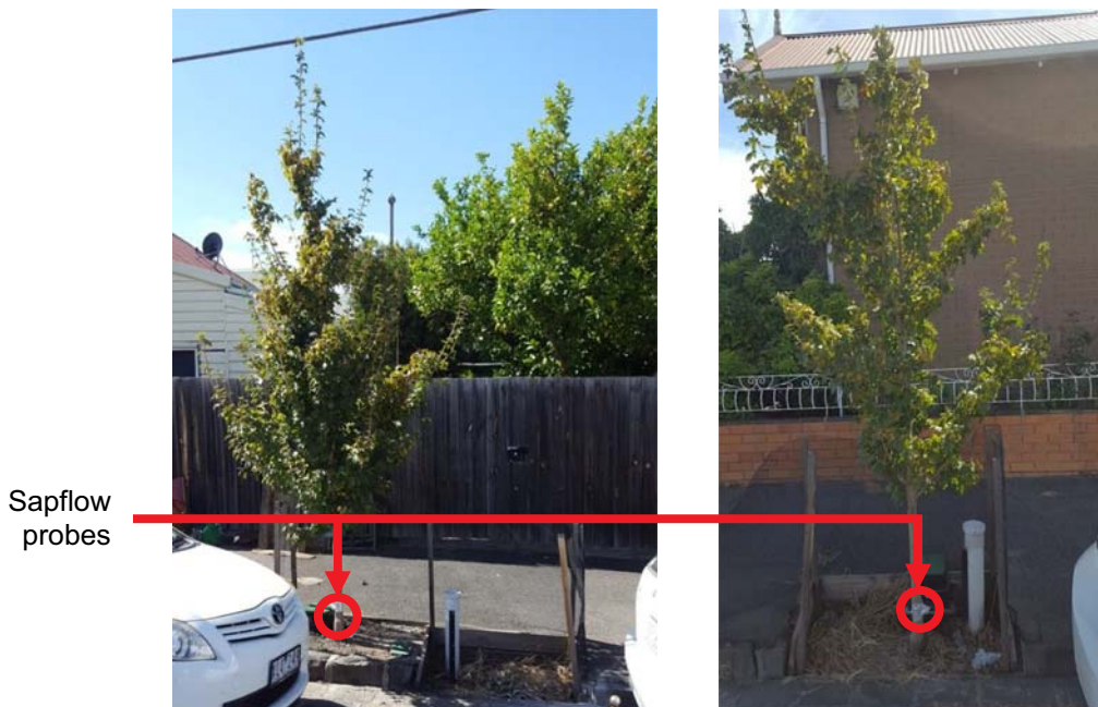
Figure 4.20 Sapflow probes used to directly measure transpiration from SCMs with establishing trees. Source: Jasmine Thom (University of Melbourne).
