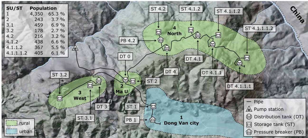
Figure 7 | Topology of the water supply system with substantial components and division of the water within the main supply areas (SU: supply unit).
